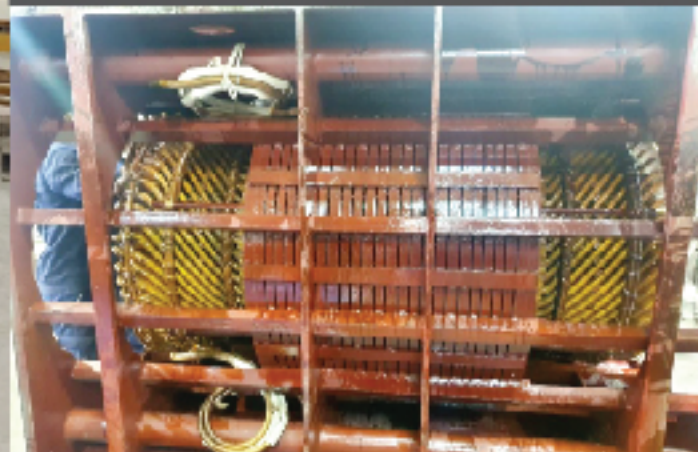
13.8 KV - 3100 KW STATOR
